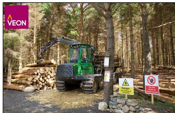
Photo 28 shows a harvesting machine felling a tree within a conifer stand. Photo 29 shows a forwarder stacking felled timber the roadside.
