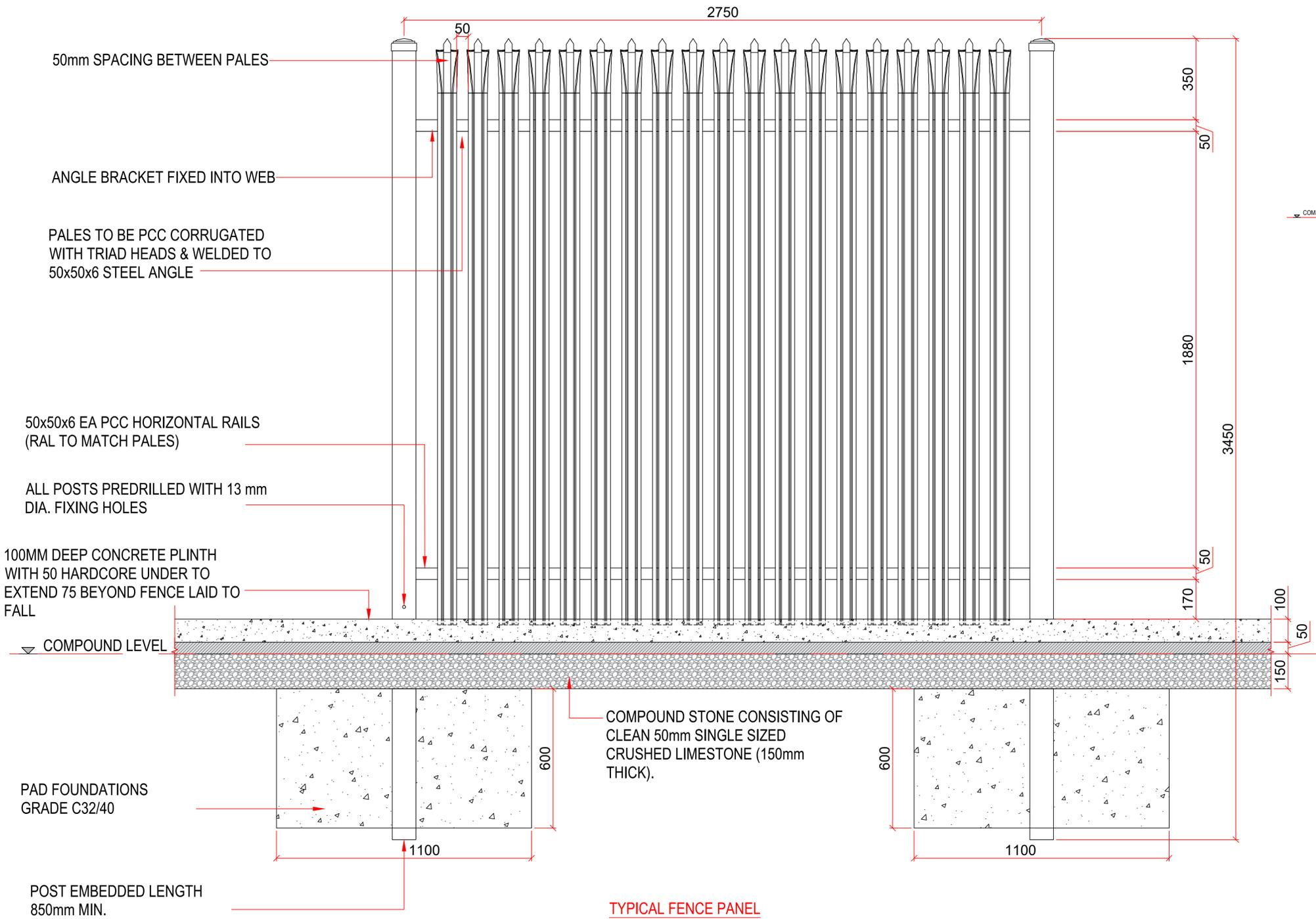
**TYPICAL FENCE PANEL ELEVATION**
