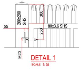
TOP OF PANELS TO GATES TO BE LEVEL WITH TOP OF PALES TO FENCE
