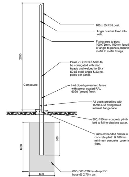
**Typical palisade fencing details - section**
