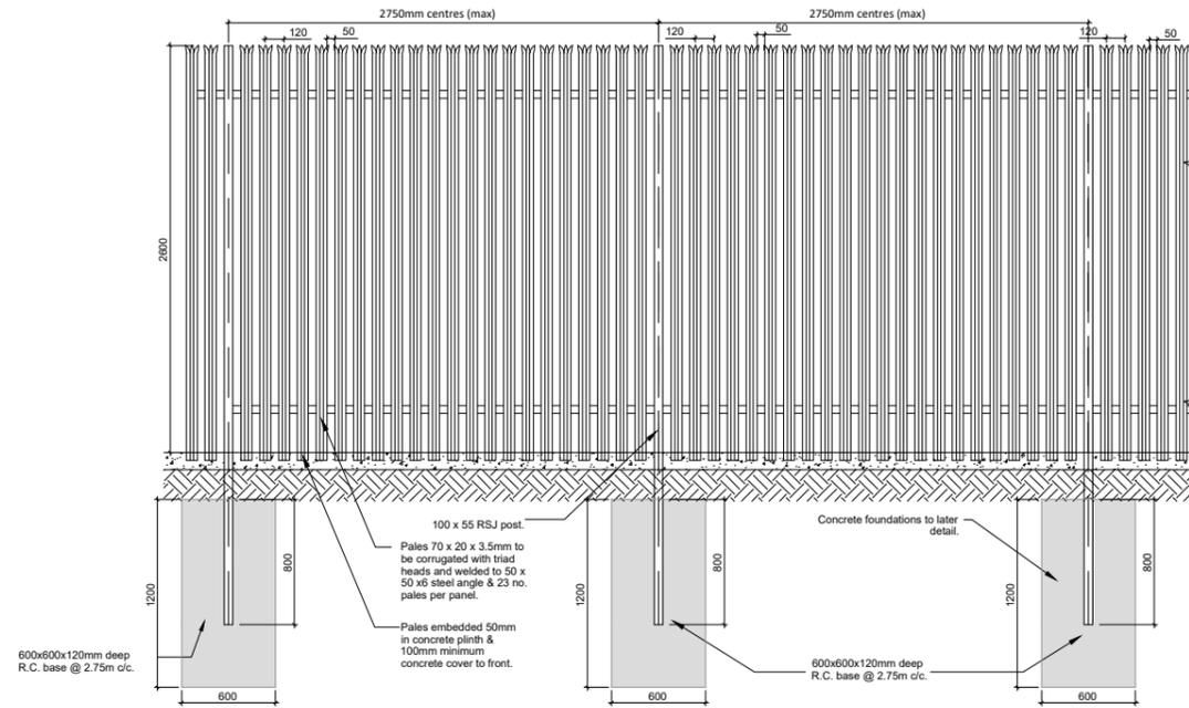
**Typical palisade fencing details - elevation**
