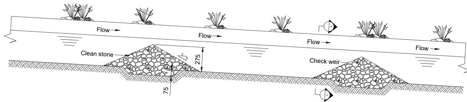
**Longitudinal section through drainage with check weirs**
