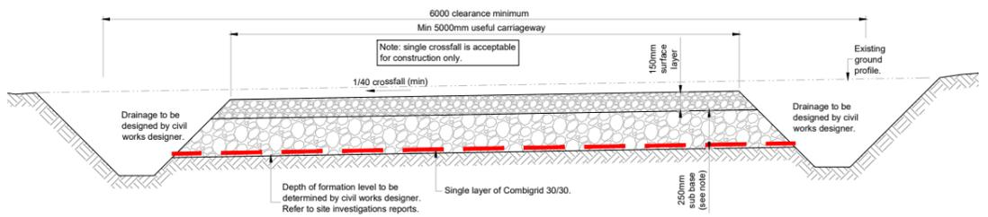
**Section through new site road construction phase (CBR between 2% and 4%)**
