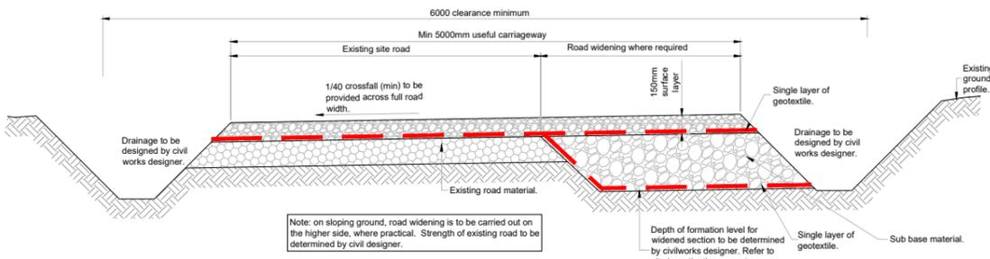
**Road widening on existing site roads where required construction phase**
