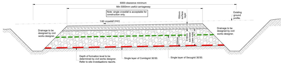
**Section through new site road construction phase (CBR between 1% and 2%)**
